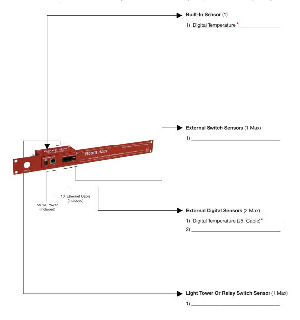
Note: The total sensor capacity of the Room Alert 4ER is 4+ sensors. Includes port for direct connection of a Light Tower or Relay Switch Sensor.
