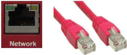
An RJ-45 port connects Room Alert 4E to your network via an RJ-45 network cable.
