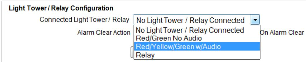
The sample screen below shows the options for a Light Tower w/Audio before it has been configured.
