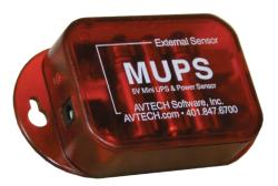
To test the Power Sensor, turn off the power source or unplug the connected power adapter. Loss of power will be recognized by the Room Alert ID Box and it will generate an alarm condition or status. A status LED will be seen when main power is present and will turn red when running on battery backup power. Managers should test the Power Sensor on a regular basis to ensure the Power Sensor is fully operational.
