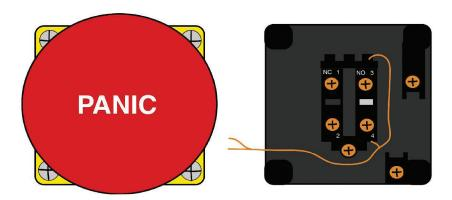
The two normally 'open' connectors in the alarm switch are wired to the Room Alert ID Box using sensor cable. The normally 'open' switch has the letters 'N.O.' printed on the switch in very small letters and is gray in color.
