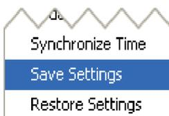
The **‘Save Settings’** feature can be used to download the current configuration settings on a Room Alert 11E unit for backup purposes. This feature can also be used to quickly configure multiple Room Alert 11E units by configuring one unit, selecting it, clicking the ‘Save Settings’ option, then selecting multiple units and clicking the ‘Restore Settings’ option.
