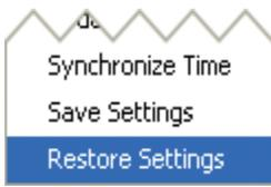
The **‘Restore Settings’** feature is used to restore a saved configuration created using the ‘Save Settings’ feature to one or multiple Room Alert 11E units. When selected, the user will need to select from a previously saved ‘.bak’ file located in the ‘log’ folder of the ‘AVTECH Device Discovery Utility’ directory in order to restore or update the settings on the Room Alert 11E unit(s).
