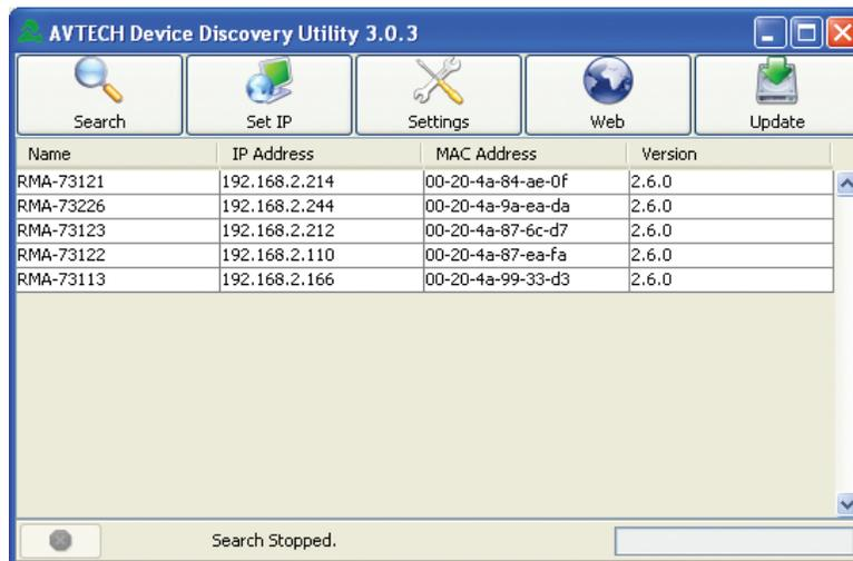
The Room Alert 11E unit connected to your network should appear in the AVTECH Device Discovery Utility window as illustrated above. This will normally take just a few seconds. If the IP address displayed is ‘169.xxx.xxx.xxx’ and the ‘Name’ is displayed as ‘Unknown’ or if the Room Alert 11E unit was not found, please see the ‘Device Not Found Or Invalid IP Address’ subsection below before continuing.
