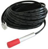
The AVTECH Digital Temperature Sensor provides a real-time digital temperature reading at the location of the temperature probe. The temperature range is from -67° to 257° Fahrenheit and/or -55° to 125° Celsius. Accuracy is within +/- 0.5 degrees. This is an instant 'plug & play' sensor that connects to one of the external environment sensor channels via an RJ-11 cable.
