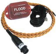
The AVTECH Flood Sensor is available with a standard 8' or 24' flood sensor cable and allows a real-time notification of flood or water leakage wherever the attached flood sensor cable is located. This is an instant 'plug & play' sensor that connects to one of the switch sensor contact sets via a low voltage 2-wire cable.
