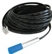
The AVTECH Digital Temperature/Humidity Sensor provides a real-time digital temperature and digital humidity reading at the location of the sensor probe. The temperature range is from -67° to 257° Fahrenheit and/or -55° to 125° Celsius. Accuracy is within +/- 0.5 degrees. The humidity range is from 0 to 100 percent Relative Humidity (%RH). Accuracy is within +/- 3.5%. This is an instant 'plug & play' sensor that connects to one of the external environment sensor channels via an RJ-11 cable.
