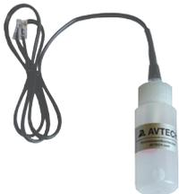
The AVTECH Digital Fluid Temperature Sensor allows real-time temperature values from -67 to 257 degrees Fahrenheit and/or -55 to 125 degrees Celsius. Accuracy is within +/- 0.5 degrees. Its non-conductive casing makes it a perfect sensor for monitoring the temperature of fluids in extreme environments, walk-in coolers, lab refrigerators or freezers. This is an instant 'plug & play' sensor that connects to one of the external Environment Sensor Channels via an RJ-11 port.
