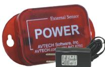
The AVTECH Power Sensor allows a real-time notification of main or UPS power status change (i.e. power going on or off). This is an instant 'plug & play' sensor that connects to one of the Switch Sensor Contact Sets via a low voltage 2-wire cable.
