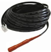
The AVTECH Digital Outdoor Temperature Sensor allows real-time temperature values from -67 to 257 degrees Fahrenheit and/or -55 to 125 degrees Celsius. Accuracy is within +/- 0.5 degrees. The external silicon coating makes the Digital Outdoor Temperature Sensor resilient enough for temperature monitoring outdoors or in other harsh environments. This is an instant 'plug & play' sensor that connects to one of the external Environment Sensor Channels via an RJ-11 port.
