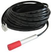
The AVTECH Digital Temperature Sensor provides a real-time digital temperature reading at the location of the temperature probe. The temperature range is from -67° to 257° Fahrenheit and/or -55° to 125° Celsius. Accuracy is within +/- 0.5 degrees. This is an instant 'plug & play' sensor that connects to one of the external Environment Sensor Channels via an RJ-11 port.
