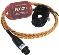
The AVTECH Flood Sensor with 24’ flood sensor cable allows real-time notification of flood/water leakage wherever the attached sensor cable is located. Water can be detected anywhere along the orange cable. This is an instant ‘plug & play’ sensor that connects to one of the Switch Sensor Contact Sets via a low voltage 2-wire cable.
