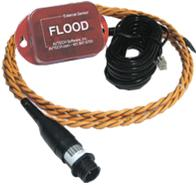
The AVTECH Flood Sensor with 8’ flood sensor cable allows real-time notification of flood/water leakage wherever the attached sensor cable is located. Water can be detected anywhere along the orange cable. This is an instant ‘plug & play’ sensor that connects to one of the Switch Sensor Contact Sets via a low voltage 2-wire cable.
