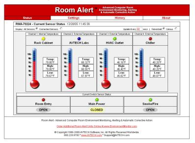
If the temperature is between the high and low thresholds and more than five (5) degrees from either threshold, the status icon will be green. If it is within five (5) degrees of the high threshold, the status icon will be yellow. If it is within five (5) degrees of the low threshold, the status icon will be blue. If the high or low threshold is exceeded, the status icon will be red. If no thresholds are currently defined, the status icon will be gray.
