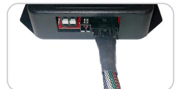
*To use your Relay Switch with the Room Alert 4E model, connect it directly to the Room Alert 4E's custom port.*
